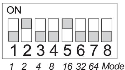
Each switch has a value - 1, 2, 4, 8, 16, 32 and 64 (the Mode switch should be left OFF). Adding together the value of switches 1-7 that are set to 'ON' sets a zone number for the control plate. The above example shows values of 2 and 16 set to 'ON' and therefore denotes Zone 18.
